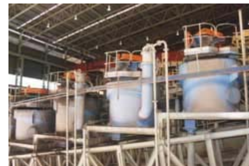
These Karee UG2 flotation cells are aligned in a configuration similar to the P9 Floatability Characterisation Test Rig.
